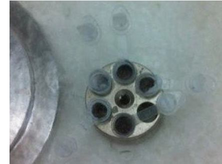
Specimen & Grid Holder for CPD and Cryo
