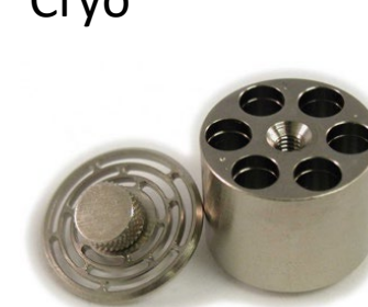
Specimen & Grid Holder for CPD and Cryo
