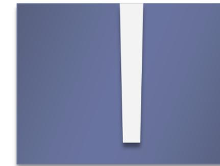
Very small positively sloped extreme high aspect ratio trench, up to 600 $\mu\text{m}$ —1 mm deep
