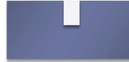
Trench ~several  $\mu\text{m}$  to hundreds  $\mu\text{m}$ , custom array of hundreds nm dia. holes
