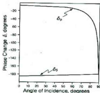
(b) Variation of phase change in the  $p$ -component and  $s$ -component radiations as function of the angle of incidence
