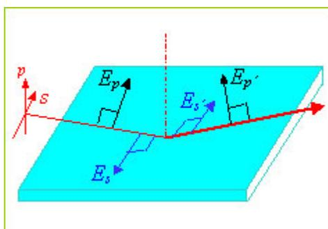
(a) Schematic illustration of the  $p$  and  $s$  polarization radiation
