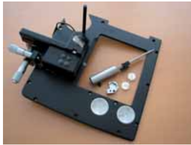
Micromanipulator for frozen hydrated sectioning
